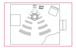
IMPORTANT: THE ROBOT VACUUM CLEANER CANNOT RETURN TO TH E CHARGING STATION IF THE STATION IS NOT CONNECTED TO THE MAINS POWER; IN THIS CASE, THE SUCTION FUNCTION WILL BE REDUCED UNTIL IT RUNS OUT AND THE ROBOT VACUUM CLEANER WILL SWITCH OFF.
