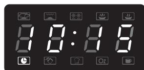
Note that when setting for am or pm, each press of the “am/pm” button will change the setting from am to pm or from pm to am.
