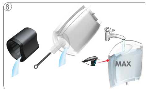
Empty capsule bin. Rinse and clean water tank thoroughly. Fill water tank with fresh, drinking water up to max. level.
