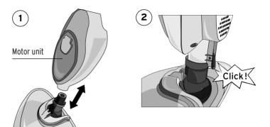
(Press lever down to remove steam head.)
