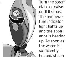
dial clockwise until it stops. The temperature indicator light lights up and the appliance is heating up. As soon as the water is sufficiently heated, steam
