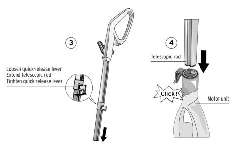
(Press button in to remove telescopic rod.)
