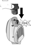
Attach the textile attachment to the bottom of the motor unit.
