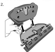
Attach the window wiper to the textile attachment.
