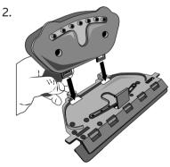
Attach the window wiper to the textile attachment.
