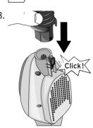
Attach the textile attachment to the bottom of the motor unit.
