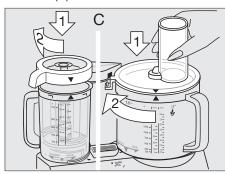
Then turn the lid clockwise guiding its nose into the safety lock opening of the motor block ① until it audibly snaps in place.
