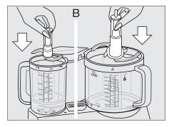
When inserting the blade @ onto the chopper bowl @, push it down until it audibly snaps in place.
