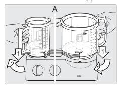
Then turn the bowl in the «function» direction until the lower fixed stop is reached. The bowl on the other drive place must be in the lifted position. If the other drive place is free, put on the protective cover <sup>®</sup>.
