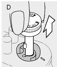
8. Allow all water to drain through the steam vents in the sole plate, while shaking the iron slightly. (Caution: Hot water and steam come out from the sole plate.)
