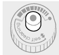
**«Extra steam»\*** (coming from the steam vents in the sole plate): For stubborn creases and wrinkles, collars and cuffs. When ironing within the red range ① area the extra steam function can be used. You can press the button ⑤ (d) for 3 seconds at intervals of no less than 15 seconds.
