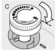
6. keep turning it to the double-arrow marking ⇄. The steam regulator will lift (C).
