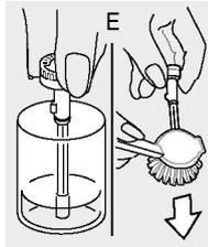
3. Then, rinse it under running water without touching the lower end of the valve.
