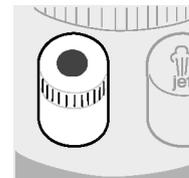
**Spray** (coming from the nozzle ③): The spray function can be used at any temperature, to dampen laundry. To do so, press the button ⑦ (water spray = blue).
