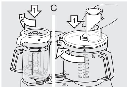
Then turn the lid clockwise guiding its nose into the safety lock opening of the motor block ① until it audibly snaps in place.
