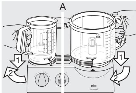
Then turn the bowl in the «function» direction until the lower fixed stop is reached. The bowl on the other drive place must be in the lifted position. If the other drive place is free, put on the protective cover ⑬.
