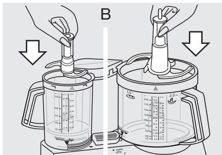
When inserting the blade ⑫ onto the chopper bowl ⑩, push it down until it audibly snaps in place.
