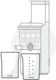
**8b** Place the **Pulp Container** below the pulp spout.
