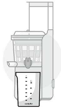
**8a** Position the **Juice Container** below the juice spout, this is on the right side of the **Juice Bowl** with the spout cover.
