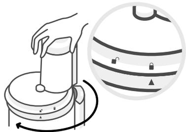
**NOTE:** To ensure the Juice Bowl Cover is fully locked, rotate it until the “locked” symbol on the Juice Bowl Cover aligns with the up-triangle symbol on the Juice Bowl (see closeup image).
