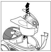
Remove the liquids/solids collection drum by pressing the catch and lifting the tank by the handle (6).
