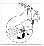
Insert the extension tube (26) onto the hose handgrip, making sure the handgrip coupling is perfectly connected to the extension tube coupling by pushing firmly together. Lock in place by rotating the locking ring (A).
