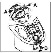
Remove the drum cover with float valve system.
