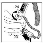
Fit the hose (25) onto the appliance. Insert the bayonet coupling (24) into the socket on the cover (1), press down and rotate clockwise as far as it will go.
