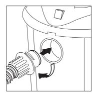
Connect the flexible hose to the inlet port of your cleaner by rotating the hose coupling clockwise until securely attached.
