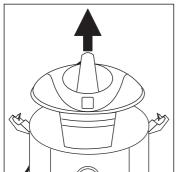
Lift off motor unit by the easy-grip handle, remove tools out of the tank and fit the tools for the task required onto your cleaner.
