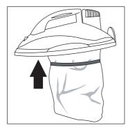
Make sure that the motor-protection paper bag is fitted over the motor housing.
