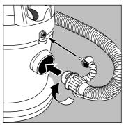
Reattach the motor unit to the tank, connect the flexible hose to the inlet port by rotating the hose coupling clockwise until securely fastened. Connect the solution dispenser (7) to the motor unit by pressing it in deeply.
