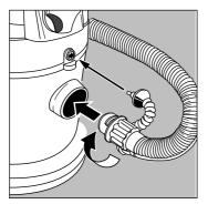
Close the port hatches, reattach the removable tank, and connect the solution injection system (10) by firmly pressing in place.
