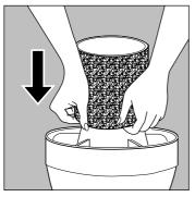
Remove the motor unit by releasing the catches (as described in "Preparing for Use"). Make sure the motor housing is fitted with the polyurethane foam filter for wet vacuum (26) and not with paper filters (27) (29) or cloth filter (28).
