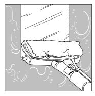
Glass can be cleaned with hot or cold water, or with steam. In all cases use the following method: spray water or steam jet on the surface to be cleaned and go over the area with the sponge side of the tool, then wipe the glass dry by turning the wiper over and using the side with the rubber scraper while vacuuming at the same time.
