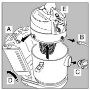
**CAUTION:** When the dirty-water tank is full, a special safety device will shut off suction automatically. At this point switch off the motor , disconnect the machine and empty the dirty-water tank.
