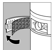
Periodically replace the exhaust filter inside the hatch on the motor unit.
