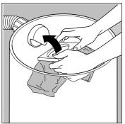
The large dustbag (29) (where provided) must be placed inside the tank by fitting the cardboard collar onto the inlet port.
