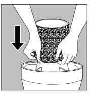
Remove the motor unit by releasing the catches (as described in "Preparing for Use"). Lift off motor unit and fit the polyurethane foam filter for wet pick up (26) over motor housing.
