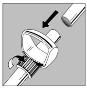
Attach one end of the extension tubes to the handgrip and the tool for the task required to the other end. If provided, the extra handgrip (30) at the tube junction will make cleaning operations easier.
