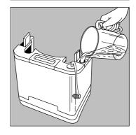
Fill the tank from the port marked with the tap symbol with plain water to the **Max** level for steam cleaning or rinsing operations.
