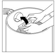
The large paper filter (35) must be placed inside the tank by fitting the cardboard collar onto the inlet port.
