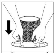
Remove the motor unit by releasing the catches (as described in "Preparing for Use"). Lift off motor unit and fit the polyurethane foam filter for wet pick up (29) over motor housing.
