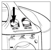
Fit the required tool to the flexible hose, plug in the power cord and switch your cleaner on by depressing the ON/OFF suction button (4) only.
