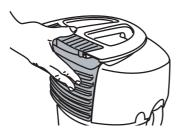
Check regularly that the float in the motor housing is free to move by raising the head of the appliance and shaking.
