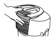
Check regularly that the float in the motor housing is free to move (fig. 11) by raising the head of the appliance and shaking.
