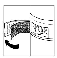
Periodically replace the exhaust filter inside the hatch on the motor unit.
