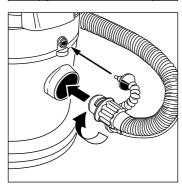
Reattach the motor unit to the tank, connect the flexible hose to the inlet port by rotating the hose coupling clockwise until securely fastened. Connect the solution dispenser (10) to the motor unit by pressing it in deeply.
