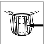
Periodically check that the float inside the motor housing is free to move in its holder.
