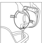
Empty the dirty-water tank with the help of the inner handle.
