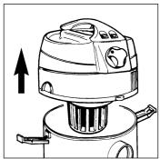
Lift off motor unit by the easy-grip handle. Remove tools out of the tank and fit the tools for the task required onto your cleaner.
