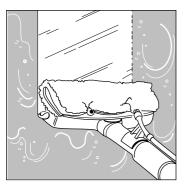
Glass can be cleaned with cold water, or with steam. In all cases use the following method: spray water or steam jet on the surface to be cleaned and go over the area with the sponge side of the tool, then wipe the glass dry by turning the wiper over and using the side with the rubber scraper while vacuuming at the same time.
