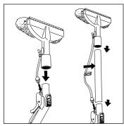
Fit the attachment either directly onto the handgrip or, if it makes work easier, use the rigid extension tubes as well.
