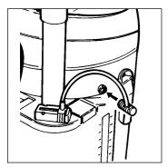
Close the port hatches, reattach the external tank in its seat, and connect the solution suction system (12) to the machine by firmly pressing in place.
