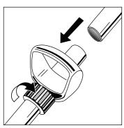
Attach one end of the extension tubes (28) to the handgrip and the tool for the task required to the other end. The extension tube handgrip (24) at the tube junction will make cleaning operations easier.
