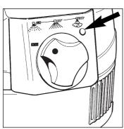
Rotate cleaning selector (6) from the OFF to the JET position and automatically a light will come on to indicate that your cleaner is ready for extraction cleaning.
