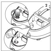
To open the boiler, unscrew the cap (fig. 2). Fill the tank with a maximum quantity of about 1.5 litres of tap water (without adding detergent).
