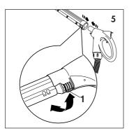
Insert the extension tube onto the hose handgrip, making sure the handgrip coupling is perfectly connected to the extension tube coupling by pushing firmly together. Lock in place by rotating the locking ring (1) (fig. 5).
