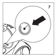
During operation, the steam ready indicator light goes on and off. This is part of normal operation.
