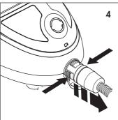
To remove, press the locking fins at the side and pull (fig. 4)
