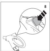
To deliver steam, hold the button on the bottom of the hose handgrip down. Release it to stop delivery. Activate suction by pressing the ON/OFF button (fig. 8). The appliance will then wash and vacuum clean at the same time.
