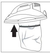
Make sure that the motor-protection paper bag is fitted over the motor housing.
