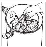
Position the dustbag inside the tank by fitting the cardboard collar onto the suction inlet port and pressing firmly in place.
