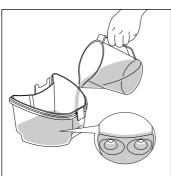
Remove the air flow conveyer (3) and pour water into the tank until the two projections on the base of the tank are covered (about 800 cc)
