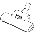
Position of selector switch for long pile rugs and carpets
