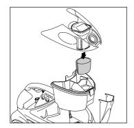
Exhaust air is filtered by a **high-efficiency filter (A)** that captures and retains particles with a size of over 3 microns. When dirty, the filter must be replaced.
