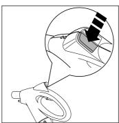
To decrease or increase suction power, press button (24) keeping it depressed until the desired suction power has been reached.
