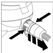
To disconnect, push on the two side locking tabs and pull.
