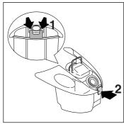
By means of the hooks, remove the tank cover with float system
