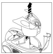
Remove the water tank by pulling the trigger and at the same time lifting the tank by the handle (6).
