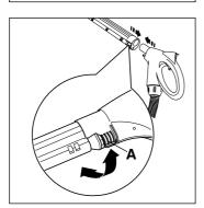
Insert extension tube (29) onto the flexible hose handgrip making sure the handgrip coupling is perfectly connected with the extension tube coupling. Push firmly all the way in, then lock into position by rotating the locking ring (A).
