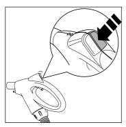
To activate vacuuming, press Suction button ON/OFF (23) on the handgrip of the flexible hose. The appliance will be reach maximum vacuuming power in a few seconds. To disactivate suction, press Suction button ON/OFF (23) once more.
