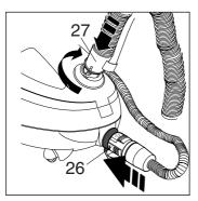
Fit the appliance with flexible hose (28). Insert bayonet coupling (27) into the hole on front cover (1), pressing it in firmly and rotating clockwise until it stops.
