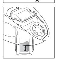
Periodically check to see that the floater is moving freely in its casing, and that wet filter (4) and air filter (7) are in place and correctly positioned in their seats.
