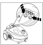
Connect the plug of the power cord to the mains, press on/off button (15) and boiler power button (16). At this point, indicator lights (17 – power) and (18 boiler on) and will come on . When the steam-ready light (19) comes on, your cleaner is ready for use.
