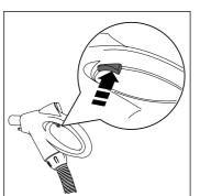
For steam output, keep button (25) under the handgrip of the flexible hose pressed and release when you want to stop steam output. Start suction by pressing the ON/OFF button (23), in this way the appliance will wash and vacuum at the same time. In case of stubborn stains, first steam and then vacuum the area (See section on "Extraction cleaning technique", p. 30.)
