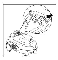
When the water in the boiler is about to run out, the water out indicator light (20) will come on. Fill the tank as follows:
