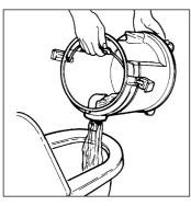
**CAUTION:** The liquid collection drum can hold approximately 8 litres of water; above this level, a special safety device will shut suction off automatically and the number of motor revolutions will increase. At this point switch off the motor, disconnect the appliance and empty the wet/dry tank.
