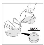
Fill the tank with water up to the maximum level marked on the tank (1,3 ltr approx).
