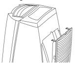
Remove the dust filter by detaching it from the grille (Fig. M). Remove 3M® electrostatic filter if it is mounted.
