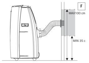
When the hose 11 is not fitted, the hole can be closed with the flange cap 10.
