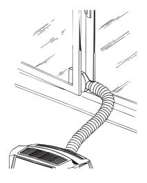
If you have a double window, use the suckers 13 provided to hold the two parts of the window together (fig. C).
