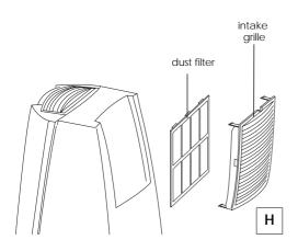
Use a vacuum cleaner to remove the dust collected on the filter.
