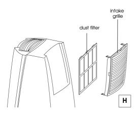
Use a vacuum cleaner to remove the dust collected on the filter.
