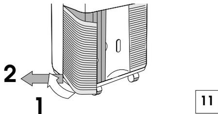
To remove the dust deposited on the anti-bacterial filter, use a vacuum cleaner. If very dirty, immerse in warm water (not more than 104° F) and rinse thoroughly. Allow the filter to dry. To replace, fit the filters to the intake grill and attach to the appliance.
