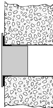
in the wall: for optimum results, insulate the section of the wall with suitable insulating material.
