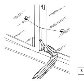
Pinguino is equipped with an adjustable window bracket. If you have a sash window, place the bracket on the window sill, extend the bracket fully within the window frame and lower the window onto the bracket. Insert the nozzle of the exhaust hose into the slot, then connect the hose to the air conditioner (Fig. 4). Thanks to the wing nut, it's possible to use the window bracket also for sliding windows. Position the hole of the bracket so to allow a correct installation of the exhaust hose.
