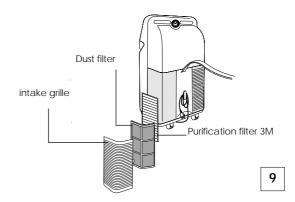
To remove the dust deposited on the anti-bacterial filter, use a vacuum cleaner. If very dirty, immerse in warm water (not more than 40° C) and rinse thoroughly.
