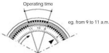
**Note:** Never turn the dial in an anti-clockwise direction!
