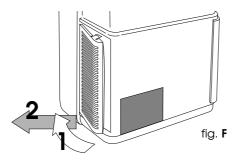
2.Remove the first air purification filter (white).
