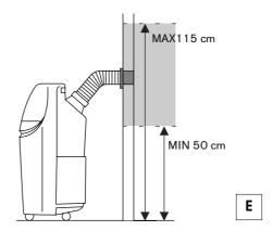
When the hose 17 is not attached, close the hole with the bung on the flange 16.
