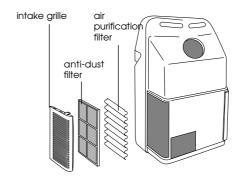
To remove dust deposited on the anti-dust filter, use a vacuum cleaner. If very dirty, rinse repeatedly in warm water at a temperature of not more than  $40^{\circ}$ C.
