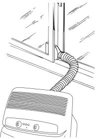
With a double casement window, use the suckers 19 provided to hold the two halves of the window together (fig. C).
