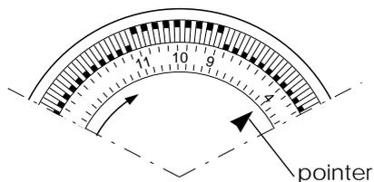
N.B.: Never turn the dial in an anti-clockwise direction!
