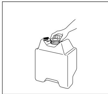
C) After completing the filling procedure, replace the extendible hose, replace the cap and screw it in tightly. Return the tank to its place, with the writing FRONT clearly visible. Carefully hold the panel in the centre and lower to its closed position.
