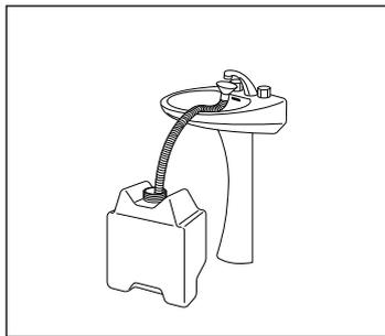
B) Turn the tank upside down and remove the plug, remove the extendible tube and fill the tank, leaving it on the ground.
