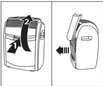
A) To open the front panel **3** grip either side of the panel and gently pull the panel towards you and upwards. Remove the tank **5** Lifting it forward.
