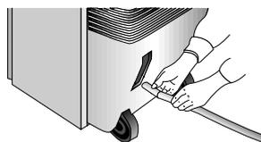
The condensation can also be drained into a basin (maximum height 11cm./4.3 ins). In this case, care should be taken to prevent overflowing.
