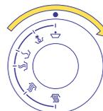
**4** Set the cooking time desired by turning the timer knob in a clockwise direction. The warning light will come on to indicate that the microwaves are working.
