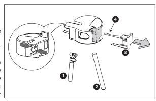
Replace the pointer, intake tube and milk spout, after making sure they are not clogged with milk residues.
