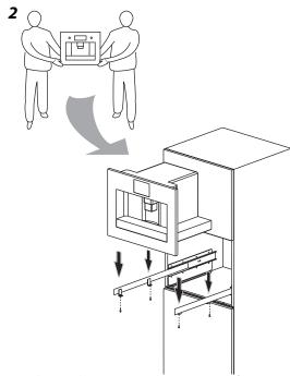
Put the appliance on its housing and fasten it with the screws.
