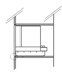
To align correctly the appliance, put the spacers under the bar's support.
