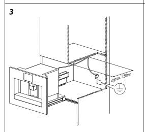
Fix the power cord with the special clip, to avoid the cord entangling when extracting or inserting the appliance.
