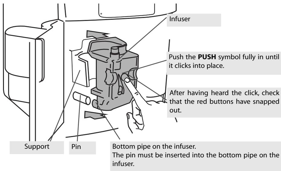
Check that the two red buttons have snapped out, otherwise the door cannot be closed..
