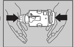
**NOTE 3:** If it is still hard to insert the infuser, leave it out of the appliance, close the service door, unplug from the mains, then plug in again. Wait for all the lights to go off after the self-diagnosis, then open the door and replace the infuser.
