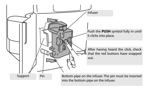
Check that the two red buttons have snapped out, otherwise the door cannot be closed.
