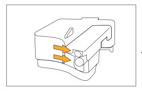
Make sure there are no milk residues inside the two holes in the lid of the milk container indicated by the arrows in the figure.
