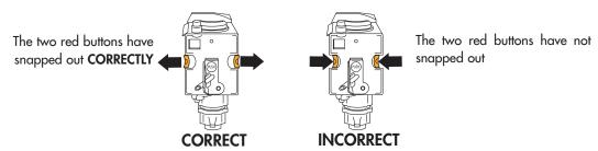
Check that the two red buttons have snapped out, otherwise the door cannot be closed.
