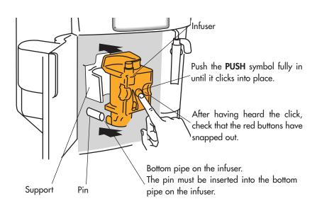
Check that the two red buttons have snapped out, otherwise the door cannot be closed.
