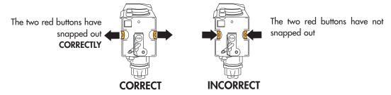
**NOTE 1:** If the infuser is not inserted correctly until it clicks into place and the two red buttons have not snapped out, the service door cannot be closed.
