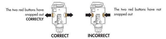
**NOTE 1:** If the infuser is not inserted correctly until it clicks into place and the two red buttons have not snapped out, the service door cannot be closed.
