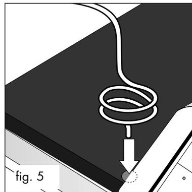
Thread the cable through the eye at the top.
