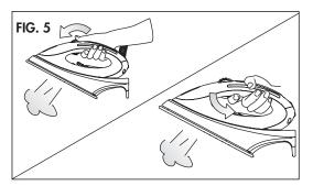
To obtain **continuous steam** rotate the wheel forwards until it locks into place.
