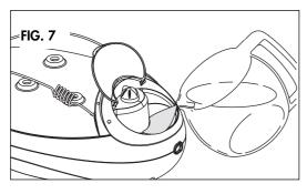
Lift the fill door (12) using the special tab. Top up until you see water appear in the filling area (fig. 7).
