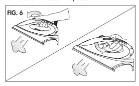
The steam regulator (8) allows the regulation of steam. The quantity of steam can be reduced or increased
