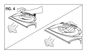
On the models where provided, the steam regulator (9) can be used to increase or decrease the quantity of steam.
