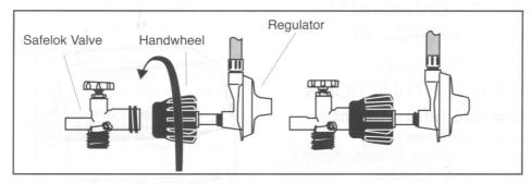
The valve on your gas cylinder should be a Safelock type and not a Clip-on, eg. Kosan type. Have your gas bottle supplier fit a Safelok valve if necessary.
