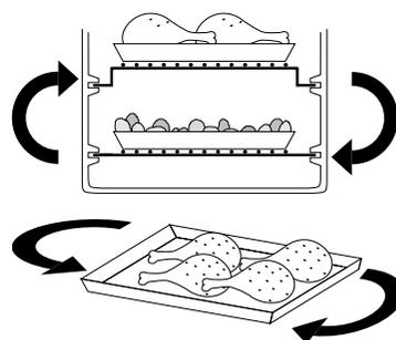
**Note: the wire racks must be positioned as shown in the figure to the side.**
