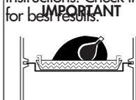
We recommend cooking chicken, roasts and small fowl directly on the broiling rack resting on the dripping-pan (see fig. on the left) to avoid fat spattering onto the sides of the oven and dripping onto the bottom. See the following sections for further details.
