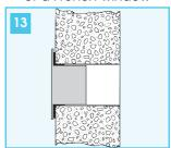
in the wall: you are recommended to insulate the section of wall using suitable insulation.
