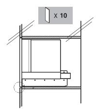
If the surface of the cabinet is not perfectly flat, place **the spacers** provided under the rail support to level the appliance correctly.
