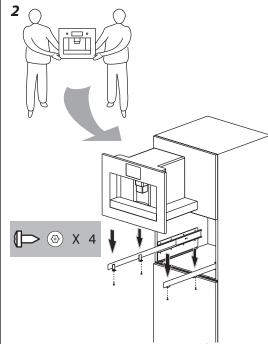
Place the appliance in the cavity and fix with the screws.
