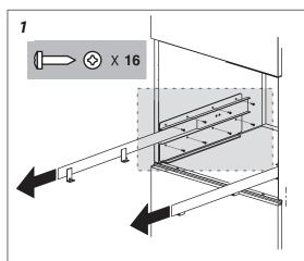
Rest the rails against the surface of the cabinet. Fix with the screws, then extract them completely.
