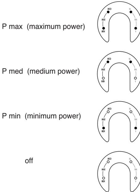
If "P max" maximum appliance operating power has been selected, adjust the thermostat dial (Fig. 2) to the desired comfort temperature, from 42°F (✱) and 95°F (5°C and 35°C).
